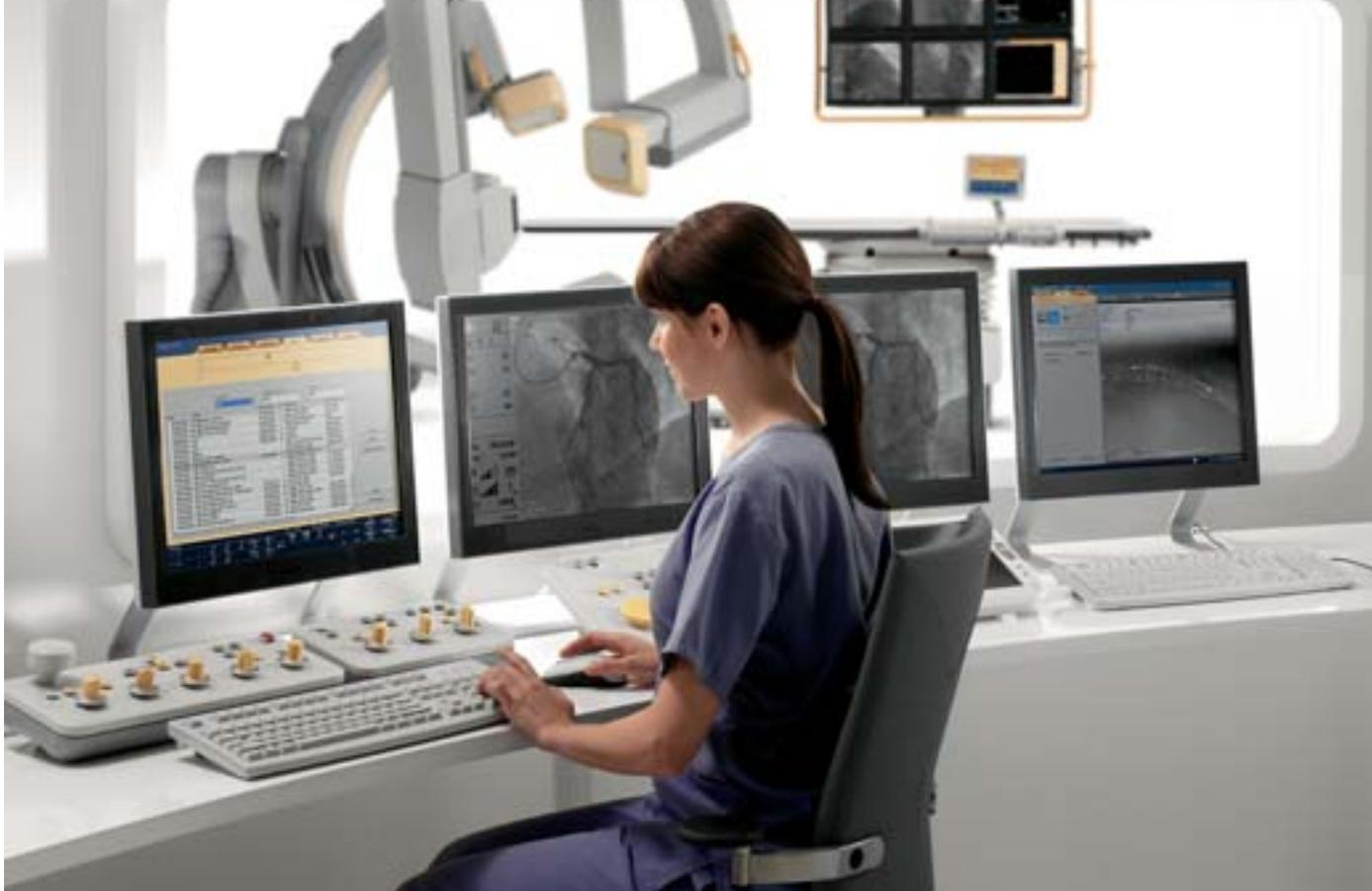
On the reference monitor, the On-Screen Display contains the user interface of the Xper ViewPad, which is used to carry out functions like run and image selection, review speed, active file selection and digital zoom.
